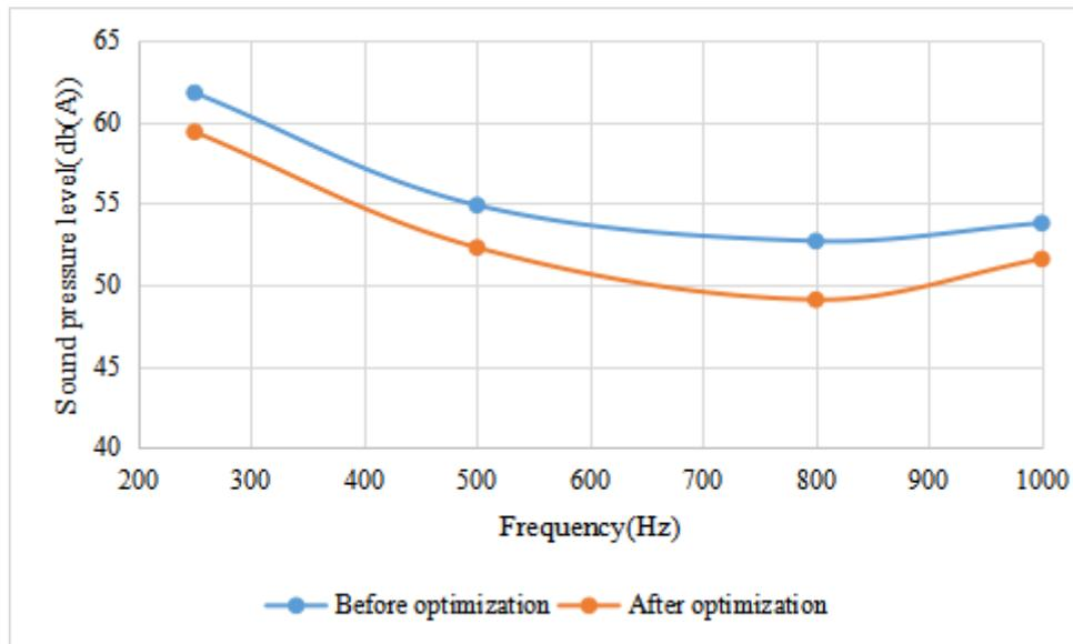
Figure 4. Comparison of sound pressure level response before and after acoustic package optimization
